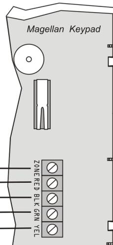
For the keypad's zone configurations, refer to the **Installer Quick Menu**. If EOL is enabled: see section [706] option [2]. Also refer to Keypad Zone Connections on page 13.
