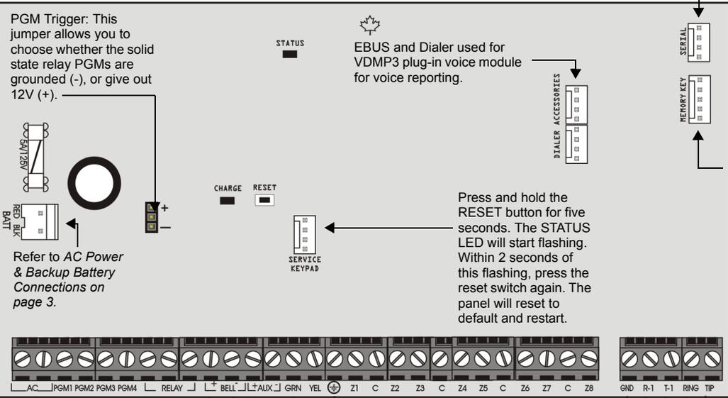
**PGM Trigger:** This jumper allows you to choose whether the solid state relay PGMs are grounded (-), or give out 12V (+).
