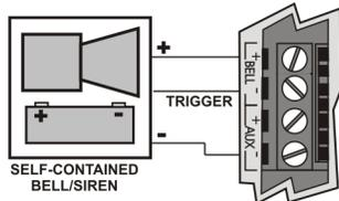
**!** The sum of the current drawn from the BELL and AUX must be limited to 1.3A (40VA transformer strongly recommended). Exceeding this limit will overload the panel power supply and lead to complete system shutdown.
